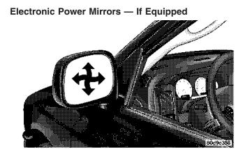
The controls for the power mirrors are located on the driver's door trim panel.
